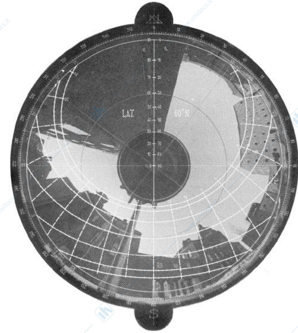
The globoscope photo combined with sun-path diagram for 60° N. latitude.
