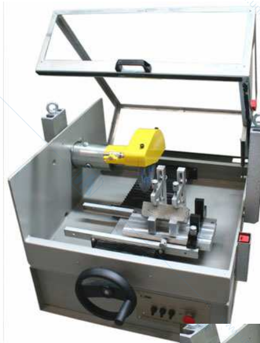
Sega circolare (core trimmer and cut-off machine)
