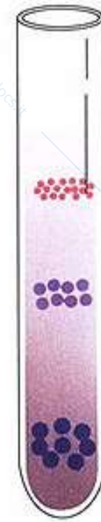
3. Gradient is formed and samples band at their isopycnic positions
