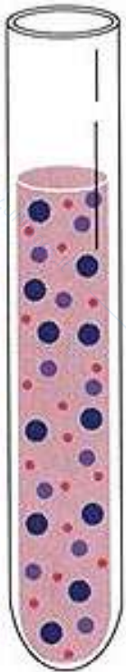
1. Uniform mixture of sample and gradient-forming substance
