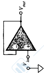
FIGURE 4.7. Voltage follower with an operational amplifier.
