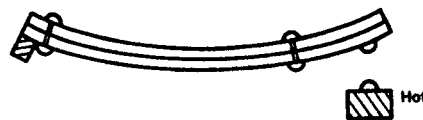
Figure 4.2 If one metal has a higher expansivity than the other, the strip will bend when heated, with the metal of higher expansivity on the outer side of the sector of the circle.
