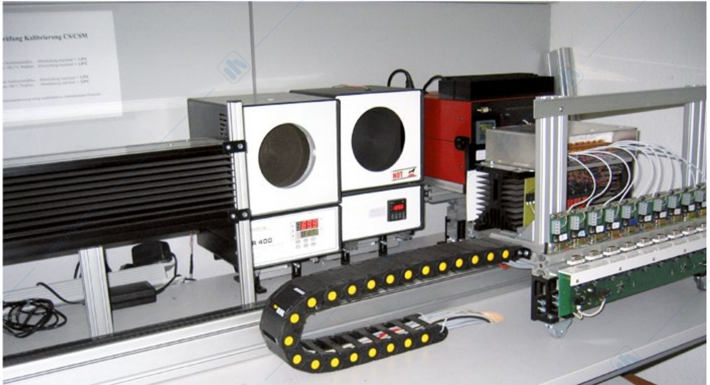
Automated calibration stations at Optris GmbH
