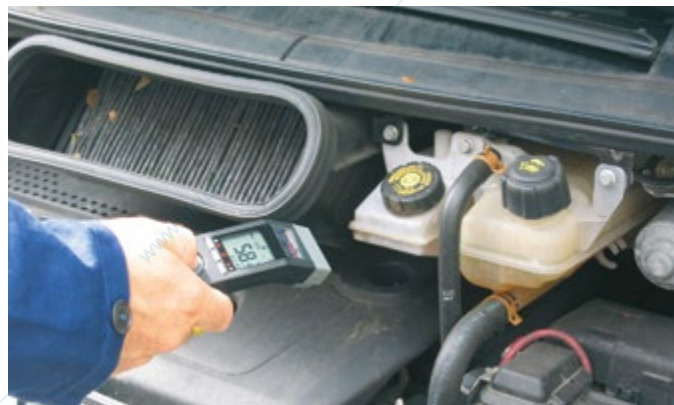
Checking the heating system
