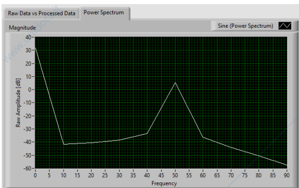
Figure 13: Power Spectrum of a Discrete Signal with 50Hz high energy spectra (LabView)
